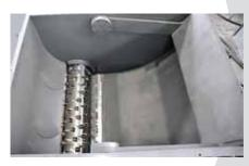
The internal ram design on the ZIS series allows the cutting chamber volume to be increased while keeping a small footprint. Making the ZIS ideal for shredding of big volume parts.
