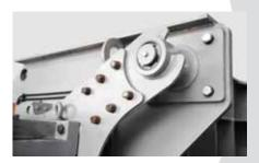
The oversized gearbox driving the rotor is supported by a very sturdy torque arm cushioning the shocks created while grinding.
