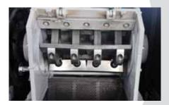
The cutting chamber sits in a soundproofed enclosure to ensure quiet inline operation. The rotor and screen area are easily accessible without for cleaning and maintenace.
