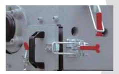
The ZERMA Quick Snap System allows the lower front plate section to be easily removed for granulator cleaning. The lower front plate section is held in position by two sturdy lever clamps.
