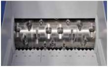
The shredders use square knives, producing high quality output. The cutters can be turned after a side is worn out.
