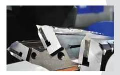
For abrasive applications the GSH granulators can be equipped with rotors with key parts manufactured from highly wear resistant steel as well as weld on hard facing.
