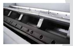
The GSH 1100 series comes standard with wide H-style rotors available with 9,11 or 13 rows of rotor blades ensuring a high quality output.
