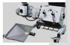
The quick snap system makes access to the cutting chamber, suction trough and screen area fast and easy. The hinged screen holder simplifies screen installation.
