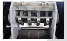
The cutting chamber sits in a soundproofed enclosure to ensure quiet inline operation. The rotor and screen area are easily accessible without for cleaning and maintenace.
