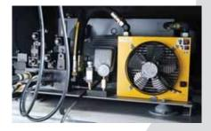
The ZXS shredders feature a high powered twin speed hydraulic system. This system ensures maximum pressure when feeding material into the rotor and high speeds on the backstroke.
