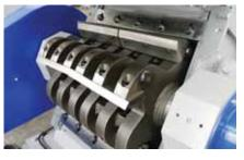
The specially angled rotor automatically pulls the fed pipes or profiles into the cutting chamber, this design also regulates the amount of material.
