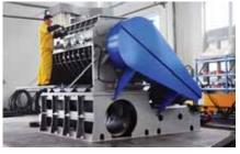
The granulators can be tailored to fit various applications, for example with oversized suction troughs in order to achieve a very high output.
