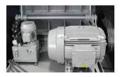
In order to keep the GSC series as compact as possible, motor and hydraulic opening system are integrated into the sound dampening enclosure of the machine.
