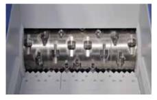
The shredders use square knives, producing high quality output. The cutters can be turned after a side is worn out.
