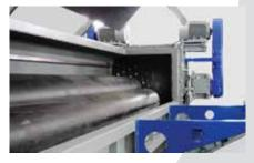
The ZRS shredders use very large diameter flat E-style rotors. The knives are fixed in special knife holders fitted in machined pockets.
