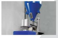
The material is fed into the Pulverizer by a vibrating dosing channel, the feeding rate is automatically adjusted based on the motors amperage and material temperature.
